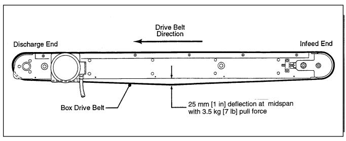
Figure 4-4 – Drive Belt Tension Adjustment (Top View)
